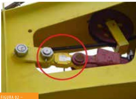
FIGURA 02 – CÉLULA DE CARGA
